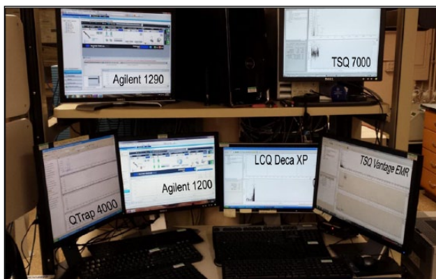
Figure 5. Data acquisition station for quadruple parallel mass spectrometry (LC1/MS4) experiment started by the partially wireless contact closure (CC) system. Instruments started from wireless CC: upper left: Agilent 1290 (Agilent Technologies, Santa Clara, CA) liquid chromatography (LC) system; upper right: TSQ 7000 (San Jose, CA) mass spectrometer; lower left: QTrap 4000 (Framingham, MA) mass spectrometer; lower center left: Agilent 1200 LC system with UV, charged aerosol detector (CAD), and evaporative light-scattering detector (ELSD); center right: LCQ Deca XP (San Jose, CA) mass spectrometer; lower right: TSQ Vantage EMR (San Jose, CA) mass spectrometer with CAD and ELSD on an SS420X analog-to-digital converter. Agilent 1290 supplying acetone dopant at 10 \mu L/min started by the Agilent 1200 autosampler for demonstration purposes, with all others performing data acquisition.
