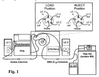
Since this used two HPLC systems and two MS systems, it was referred to as an LC2/MS2 configuration. Polar lipids were analyzed by ESI-MS, MS/MS and MS<sup>3</sup>, while neutral lipids were detected using APCI-MS and MS/MS. Dual parallel MS techniques have recently been reviewed (6,7).
